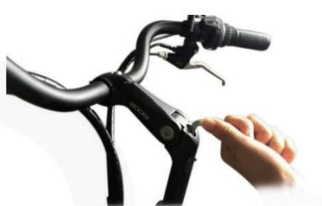
5. Adjust the tilt of the handlebar to a comfortable position ranging from  $40^{\circ}$  to  $-10^{\circ}$ , then tighten with socket head wrench.
