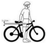
To determine the correct height for bicycle. Straddle bike, keeping feet shoulder width apart and flat on the ground. There should be a 1 - 2 inch clearance between the rider's crotch and the frame of the bike.
